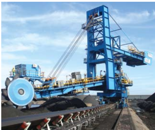
Newly commissioned combination bucket wheel stacker reclaimer at the Grindrod Matola coal terminal, Mozambique.
