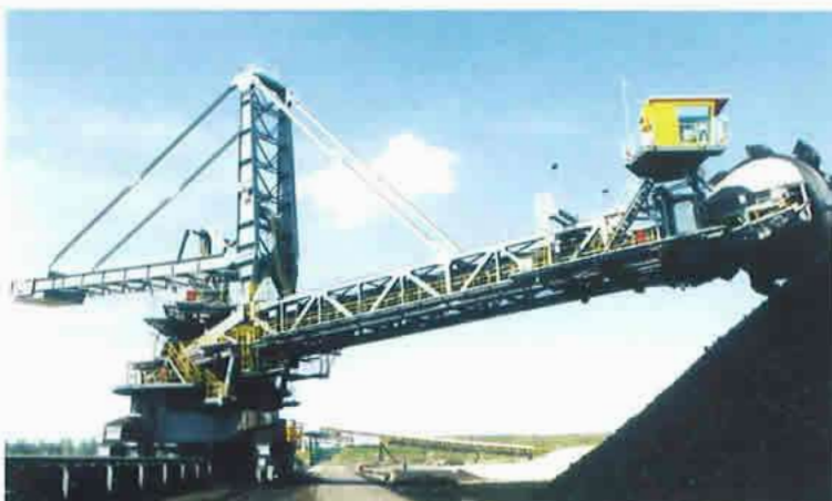
Combined bucket wheel stacker re-claimer operating in fine coal – installed in Germany.
